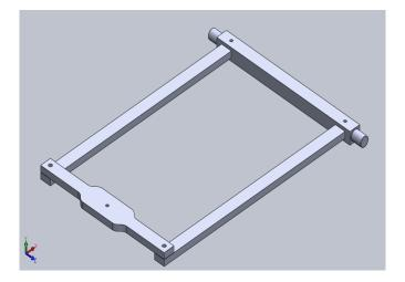
Install leveling system assembly onto chamber interface assembly per assembly instructions
