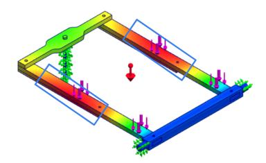
Install 2.5 kg masses at the four pendulum mounting points on the leveling system longitudinal struts (p/n-LSLS1) indicated by the purple arrows below to simulate maximum loading of the test stand pendulum assembly
